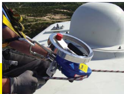
Position wheel towards you. Remove bracket if possible.
